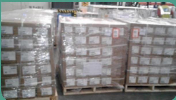
Before: Pallet with corner boards & stretch wrap
